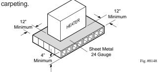
Hollow concrete cinder block; align holes and leave ends open. Alternative method for providing a non-combustible base.
